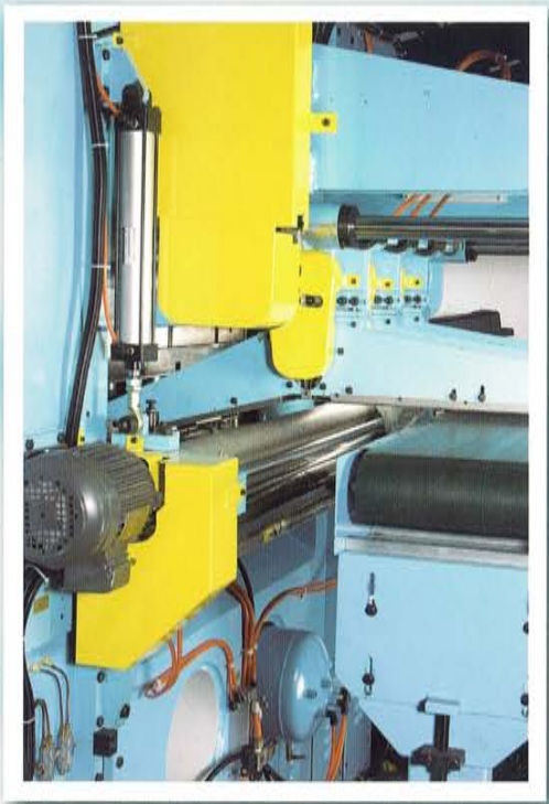
罐蓋出口輸送機及排廢料滾輪 End Discharge Conveyor and Scrap Ejector
