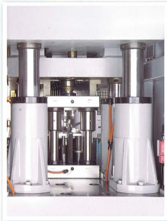
沖模側向入口及雙滑塊 Tooling Entrance and Dual Rams
