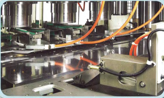
送料夾及1st引伸沖模 Sheet Clips and 1st Drawing Tooling
