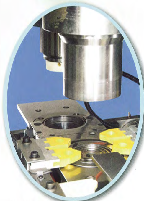
2nd 引伸冲模及修邊模 2nd drawing tooling and trimming tooling
