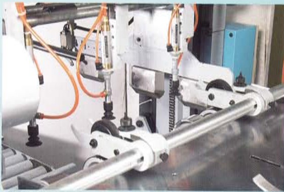
鐵皮分離器與吸盤 Sheet separator and suction pad
