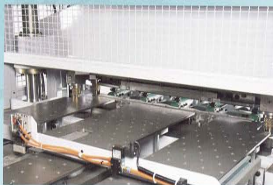
沖頭導柱與波型刀組 Ram posts and scroll blades
